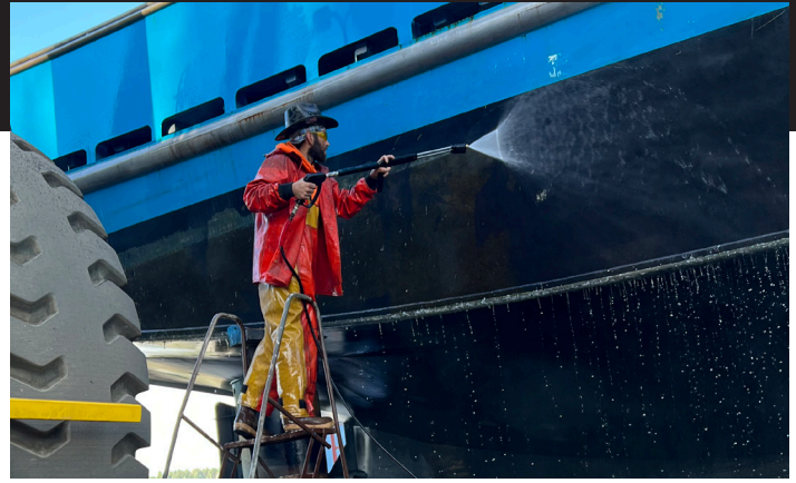
Cleaning a ship's hull is only one of the many applications for the MPE high-pressure washers with cleaning power of 5.0 GPM and 5000 PSI.
